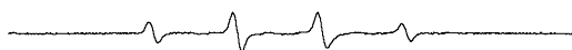
Figure 1 EPR spectrum of DMPO-OH adduct formed in the presence of Gt factor, cellobiose, Fe 3+ and O 2 .
