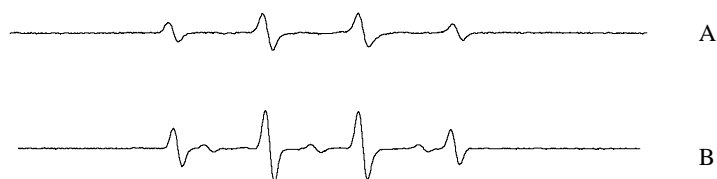
Figure 3 EPR spectra of DMPO-OH adduct obtained from Gt factor, cellobiose, Fe 3+ and O 2 . (A) spectrum from Gt factor, cellobiose, Fe 3+ and O 2 ; (B) After addition of additional Gt factor.
